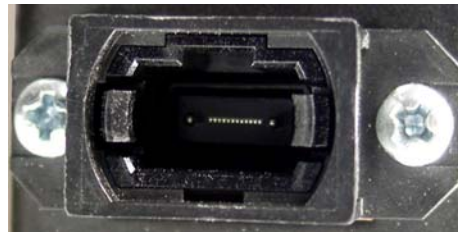
MPO adapter shown with connector installed inside the cassette
